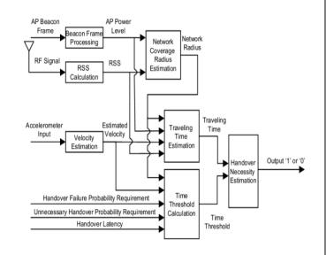
Fig. 3. Block diagram of Handover Necessity Estimation [11].
