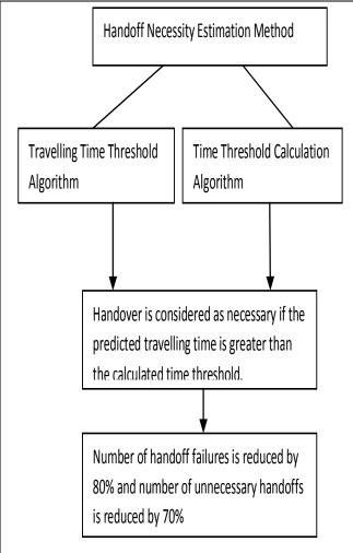
Fig. 5. Steps of Handover Necessity Estimation Method.
